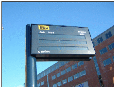
Informational displays at major stops let passengers know when their bus will be arriving.
